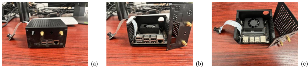
图 6 嵌入式设备 NVIDIA Jetson Xavier NX ((a)整体外观; (b)内部结构; (c)俯视图)
