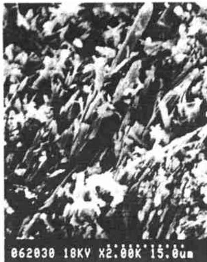
图1 K-Na 透闪石成纤维交织结构 Fig.1 SEM(secondary electron images) showing fibrous interlocking textures of K-Na richterite
