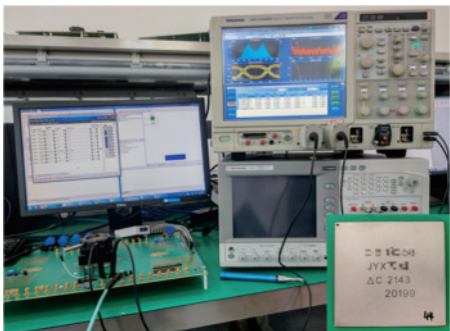
图10 LVDS驱动器测试评价系统 Fig.10 Test evaluation system of LVDS driver
