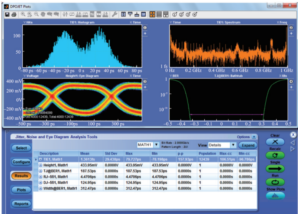
图11 测试芯片LVDS驱动器的传输特性图 Fig.11 Transmission characteristic diagram of LVDS driver in test chip
