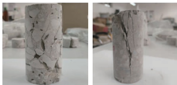
(a)Single and triaxial compression test specimens
