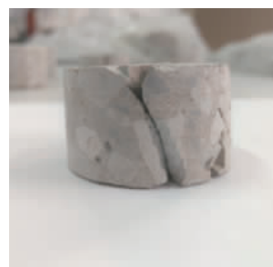
(b)Brazil splitting test specimen
