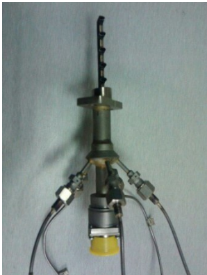
图6 级间测量探针 Fig.6 Inter-stage measuring probe
