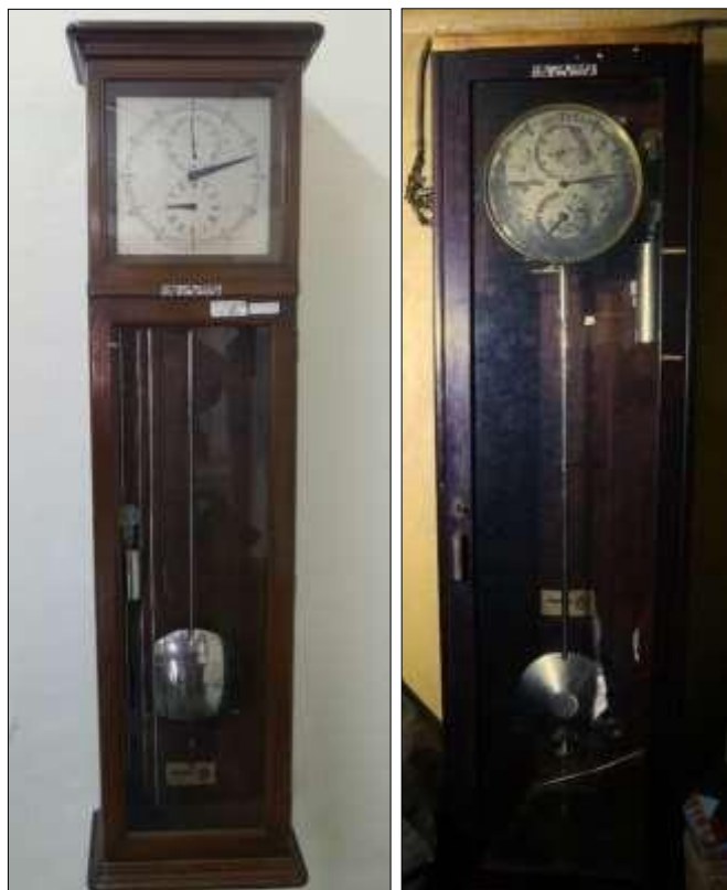
Figure 10: The Richter clock (left) is used to keep a mean time, while the Riefler clock (right) is used to keep a sidereal time. Both clocks are now placed in the Exhibition Room of the Bosscha Observatory (photographs: the authors).
