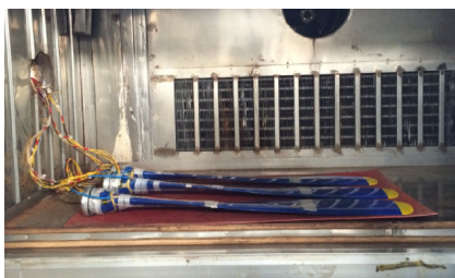
Fig. 2 Thermal test of the blade after modification
