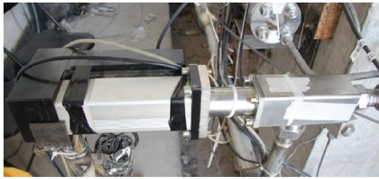
Fig. 11 Object pictures of the variable area cavitating venturi
