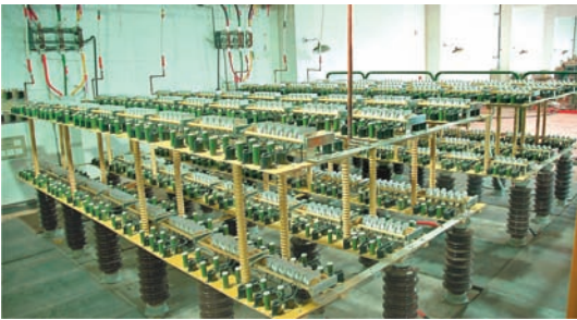
图 5 55 kV/150 A 高压直流阀体实物 Fig. 5 Picture of the 55 kV/150 A high voltage rectification valve
