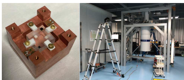
图 8 地面测试用晶体量热器模块(左图)和测试系统(右图) Figure 8 Bolometer module for ground test (left) and cryogenic system (right).
