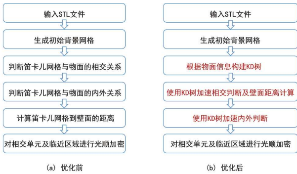
图 3 (网络版彩图)自适应笛卡儿网格生成优化前(a)和优化后(b)流程比较 Figure 3 (Color online) Comparison of processes before (a) and after (b) optimization for adaptive Cartesian grid generation.
