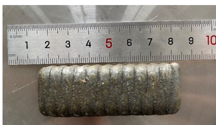
图2 激光熔覆层宏观形貌 Fig.2 Macromorphology of laser cladding layer
