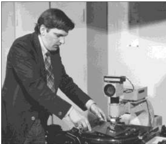
Figure 11: Here I am positioning a 10 \times 10 -inch photographic plate from the Palomar 48-inch telescope on the plate holder of the Astroscan of Leiden Observatory. The instrument scanned predefined areas with square pixels of 30 microns (corresponding to 2 arcsec on the sky) on a side (From my private archives).
