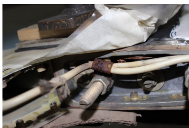
图4 旋翼内部导线包铁锈蚀 Fig. 4 Rotor internal wire wrapped iron corrosion
