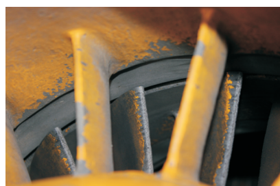
图8 风扇叶片前缘脱漆 Fig. 8 Depainting of fan blade leading edge
