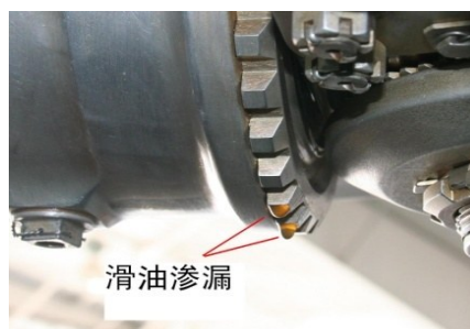
图14 旋翼关节轴承磨损 Fig. 14 Rotor joint bearing wear
