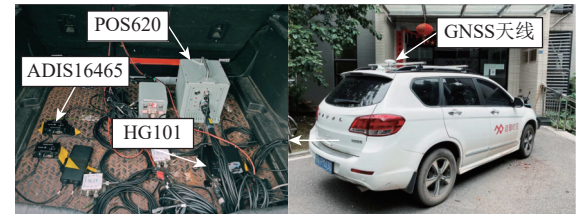
图 3 车载实验的设备安装图 Fig. 3 Equipment installation of vehicle test
