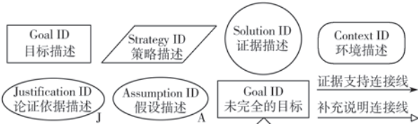
图 1 GSN 中各元素图形表示和描述 Fig.1 Graphic representation and description of elements in GSN
