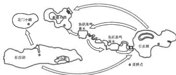
图 1 园内各湖体之间的调水示意图 Fig.1 The schematic diagram of water transfer between the lakes
