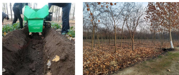
图1 安徽省六安市某地苗圃机械开沟施用污泥示意 Figure 1 Schematic diagrams of mechanical ditching and sludge application in a nursery, Lu'an, Anhui Province
