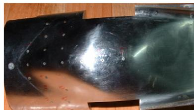
Fig. 4 Photo of bump surface on the inlet model
