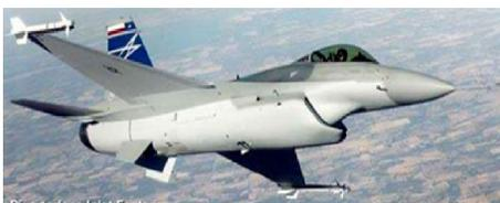
Fig. 1 F-16 validate fighter plane (diverterless supersonic inlet configuration)
