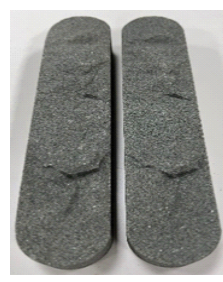
图 3 雕刻制作的砂岩岩样 Fig. 3 Sandstone sample made by carving
