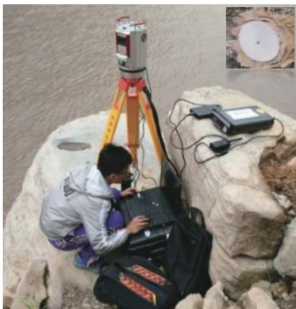
图 4 箭穿洞扫描测站及反射片 Fig. 4 Jianchuandong scanning station and reflector
