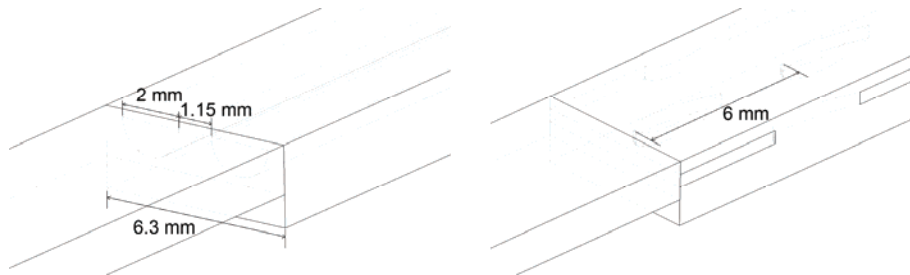
图2 印刷电路板换热器连续肋片与非连续肋片模型几何参数 Figure 2 Simulation models of PCHE with continuous and discontinuous fins
