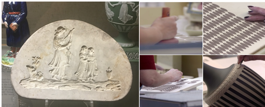
图5 浮雕玉石系列石膏模具与浮雕制作工艺图 Fig.5 Plaster mould for Jasperware and carving process of bas-relief
