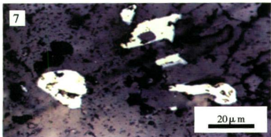
图版 7 它形粒状黄铜矿(黄色)半包裹半自形的黄铁矿(亮黄色)反射单偏光 Plate 7 Shaped granular chalcopyrite (yellow) half-wrapped semi-euhedral pyrite (bright yellow). reflect a single polarizer
