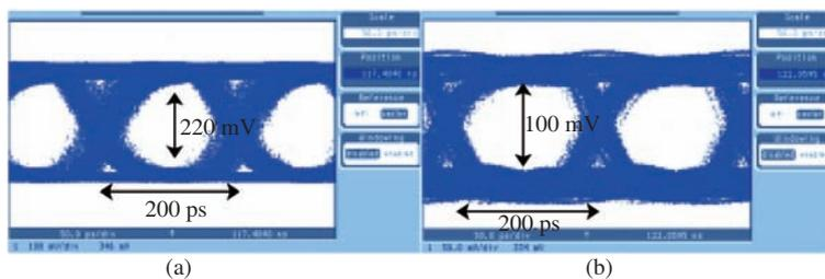
**Figure 15** Measured 10 Gb/s/pin data eye diagram: (a) 5 Gb/s RF (25 GHz RF carrier); (b) 5 Gb/s BB.
