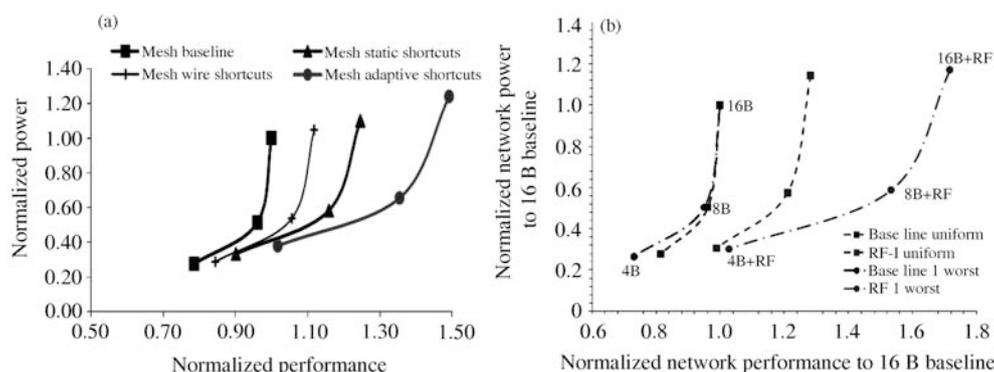
**Figure 10** (a) Power performance trade-off curve of the mesh adaptive shortcuts over the mesh baseline; (b) power performance trade-off curve on different baseline mesh bandwidth from 16 Byte wide to 4 Byte wide baseline mesh.
