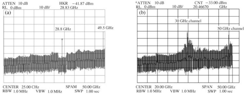
**Figure 8** Spectrum on the differential mode RF-I signal with (a) no data input; (b) with 4 Gbps data input in each band.
