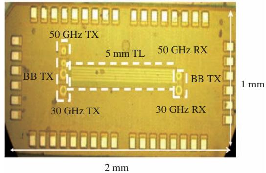
**Figure 6** Die photograph of the tri-band on-chip RF-I based on 90 nm IBM CMOS.
