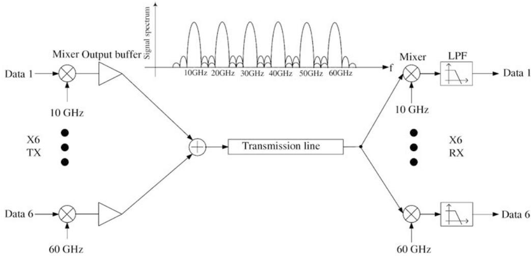
**Figure 4** Conceptual schematic of the multi-band RF-interconnect with six RF carriers.
