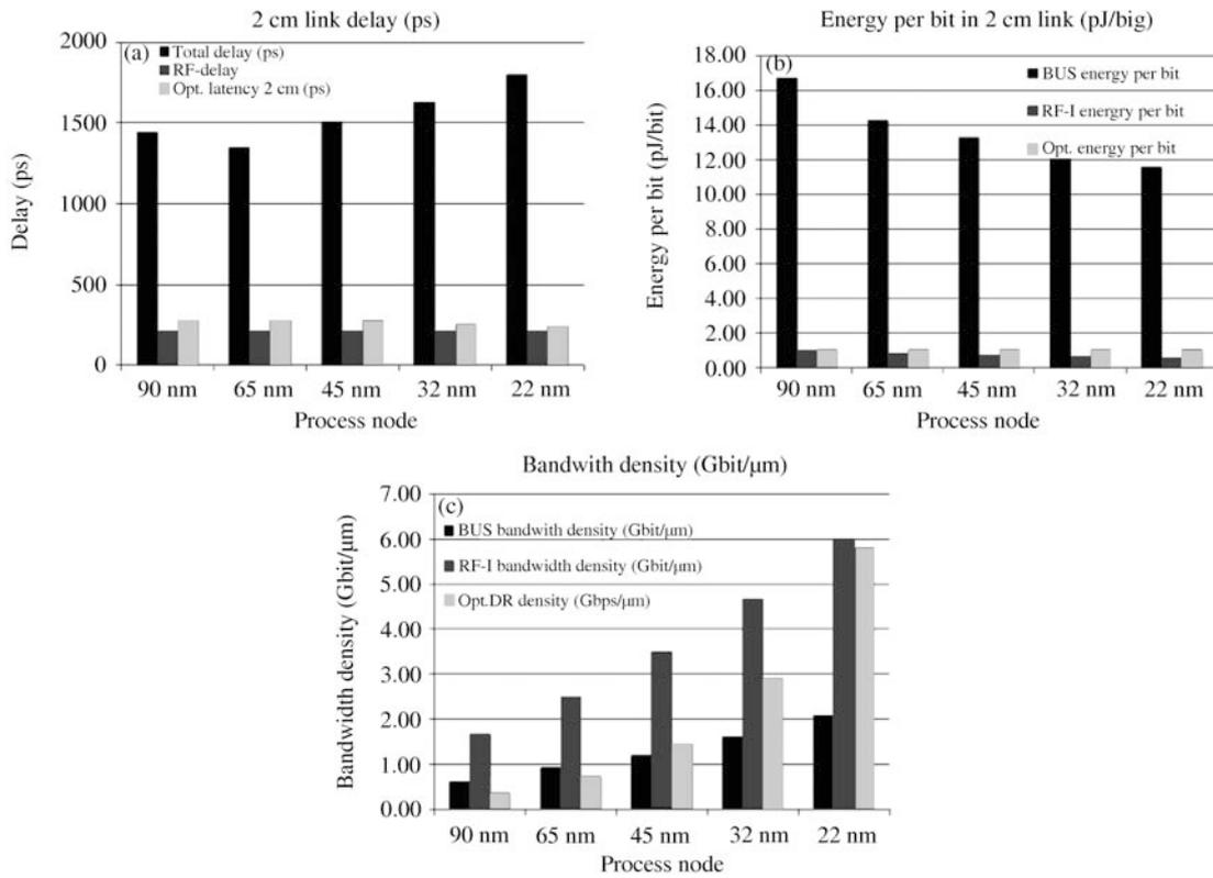
**Figure 18** Comparison of interconnect technologies for a global 2 cm (a) on-chip distance of latency, (b) energy consumption per bit and (c) data rate density for a traditional repeated parallel bus, RF-I and optical interconnect.
