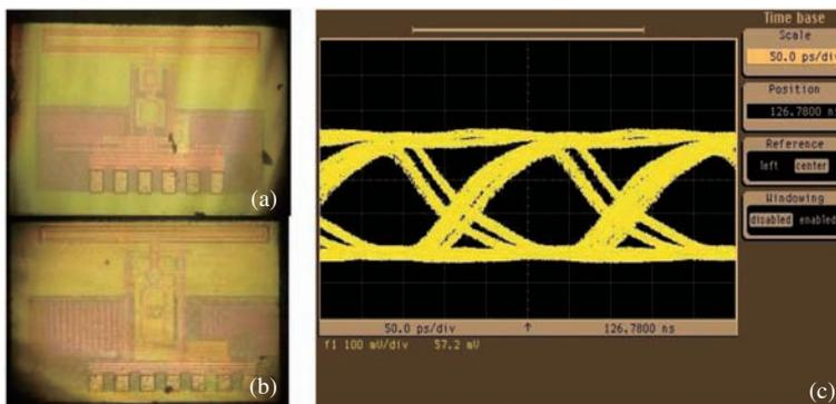
**Figure 17** (a) and (b) Chip microphotograph WRF-I transceiver; (c) measured 5 Gb/s/channel data eye diagram.
