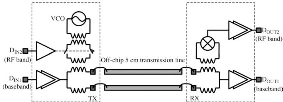
**Figure 13** Schematic of the advanced RF-I memory interface system.
