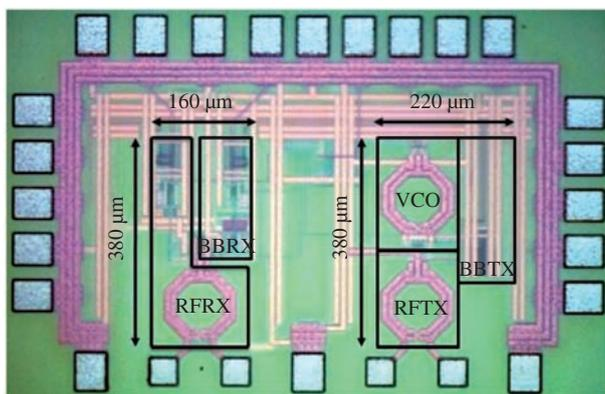
**Figure 14** Chip microphotograph of the advanced RF-I memory interface system.
