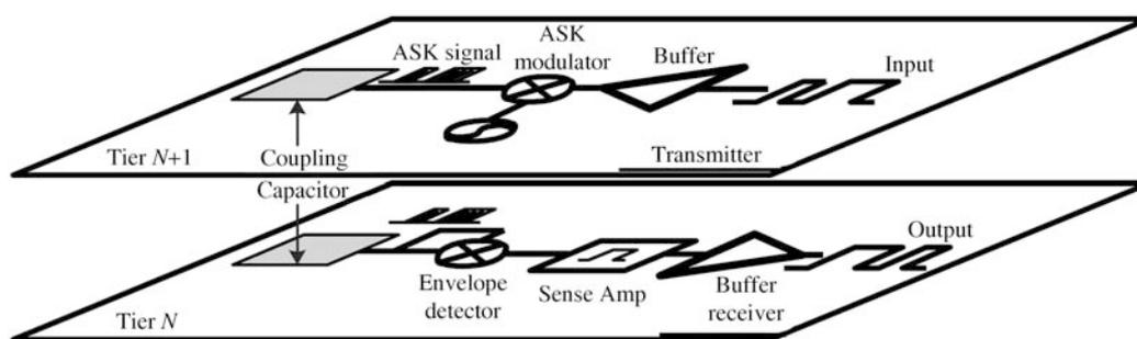
**Figure 11** Schematic of the RF-interconnect implemented in a 3D 0.18  $\mu\text{m}$  CMOS process.
