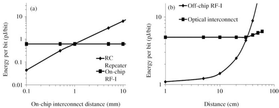
**Figure 19** (a) RF-I will crossover the energy efficient curve of the RC repeater, and become more energy efficient above a 1 mm interconnect distance at a 16 nm CMOS process; (b) RF-I has much better energy efficiency in the mid-range distance of 30 cm or below, while the optical interconnect does not have any benefit until an interconnect distance over 30 cm.
