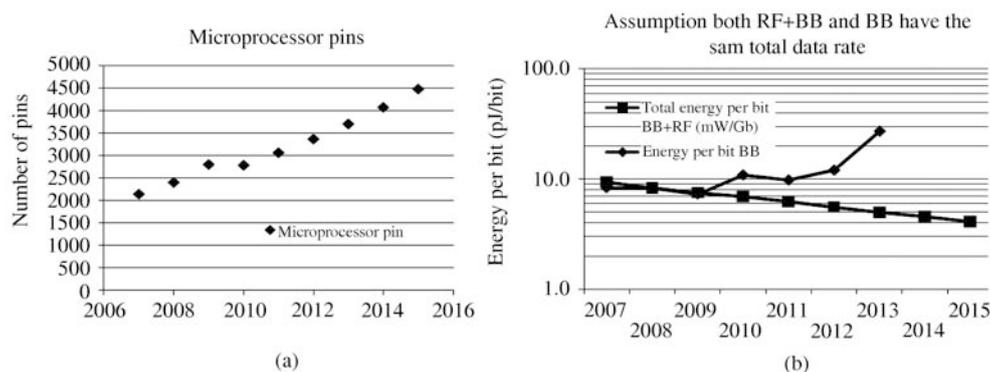
Figure 3 (a) Slow I/O pins scaling in microprocessor; (b) non-scalable energy per bit in off-chip baseband (BB) interconnect.
