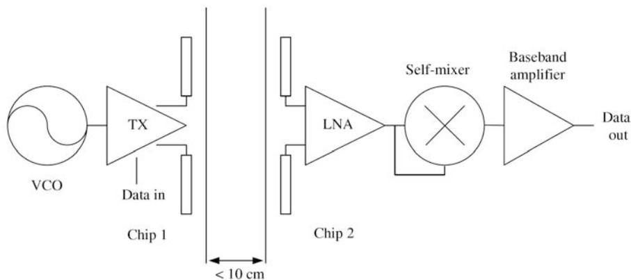
**Figure 16** Schematic of a single channel wireless RF-I using on-chip antenna.
