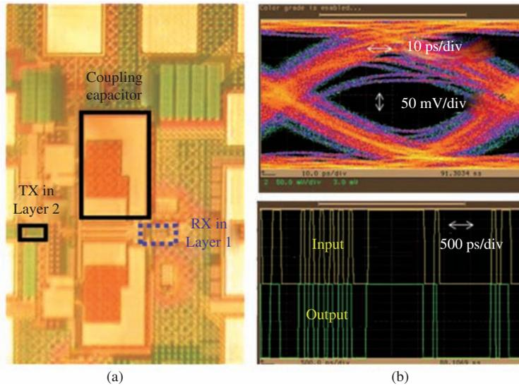
**Figure 12** (a) Chip photograph of 3D RF-interconnect; (b) measurement result of the 3D RF-Interconnect at 11 Gbps with  $2^{15}-1$  PRBS.
