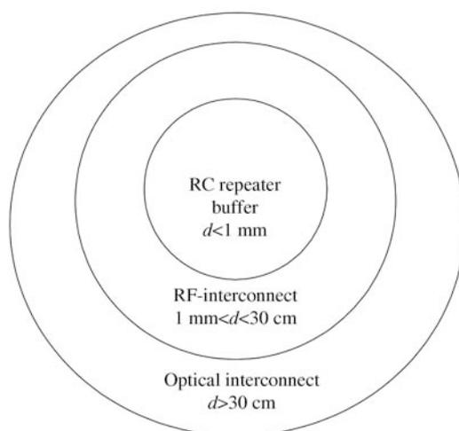
**Figure 20** Communication range versus interconnect technologies as CMOS process continuously to scale toward 16 nm.
