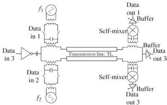
**Figure 5** Schematic of the on-chip tri-band ASK RF-I.
