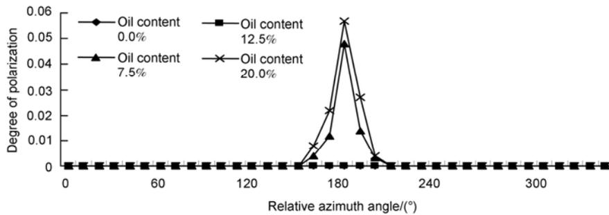
**Figure 4** The polarization degree of reflected light of the soil with 0.0% water content at 50° incidence zenith angle and 10° viewing zenith angle.
