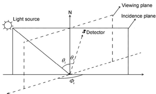
**Figure 1** Measurement geometry.  $\theta_i$ , incidence zenith angle;  $\theta_v$ , viewing zenith angle;  $\phi_r$ , relative azimuth angle.
