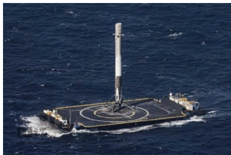
图1 猎鹰-9火箭一子级成功完成海上平台回收试验 Figure 1 The first stage of Falcon 9 Rocket flight back and landed on ASDS
