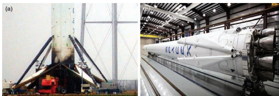
图9 猎鹰-9火箭着陆缓冲支架。(a) 展开状态; (b) 收拢状态 Figure 9 Landing legs of Falcon 9 rocket. (a) Deployed; (b) undeployed
