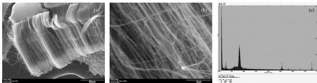
Figure 4. SEM images of raw MWCNTs-Fe (a); Pt-Fe/MWCNTs (b) and its EDS spectrum (c)
