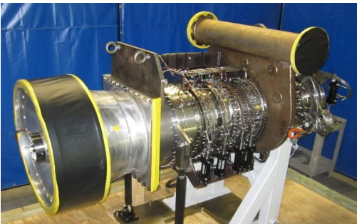
图5 自由工厂参与的 HEETE 压气机试验件 Fig.5 HEETE compressor test rig which LibertyWorks was participated
