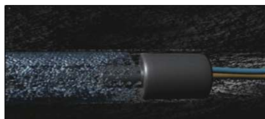
(b) 喷涂式封孔孔内原理
