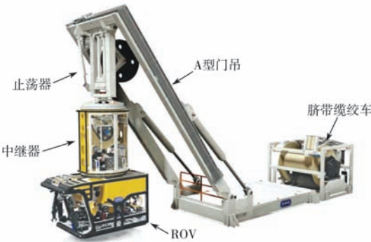
图 4 作业级 ROV 系统组成结构 Fig.4 System structure of work-class ROV
