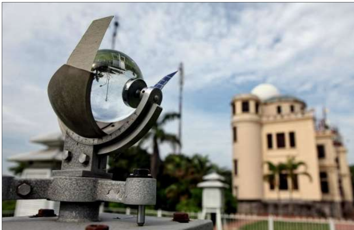
Figure 15: A Dutch pyrliometer, used to measure sunlight, set up in the meteorological precinct at Phù Liễn Observatory (courtesy: Phù Liễn Observatory).
