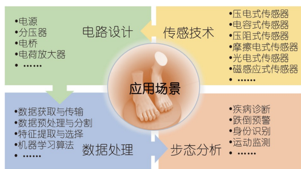
图1 (网络版彩色)用于步态分析的足底压力监测系统概述 Figure 1 (Color online) Overview of the plantar pressure monitoring system for gait analysis
