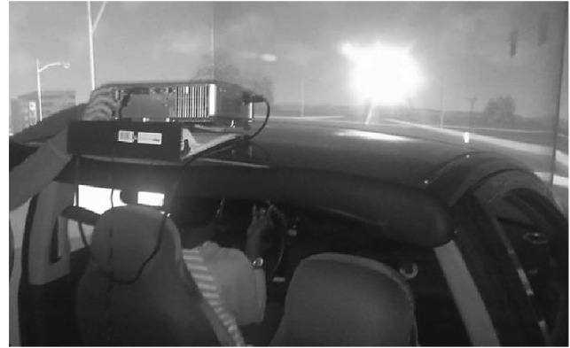
Fig. 1 – Driving simulator at an intersection with sun glare.
