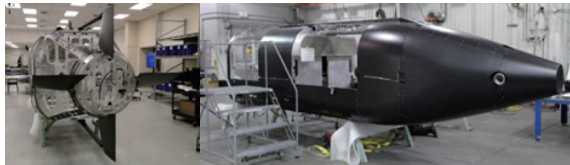
图 4 MK 11 湿式蛙人输送艇原理样机尾段结构 Fig. 4 Principle prototype tail structure of wet diver delivery vehicle (MK 11)
