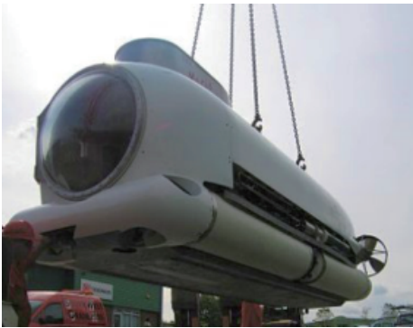
图 11 干式蛙人输送艇 UOES1 Fig. 11 Dry diver delivery vehicle UOES-1
