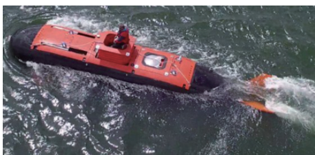
图 12 干式蛙人输送艇 UOES-2 Fig. 12 Dry diver delivery vehicle UOES-2
