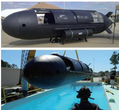
图 5 多功能双模蛙人输送艇 PROTEUS Fig. 5 Multi-function dual mode of diver delivery vehicle PROTEUS
