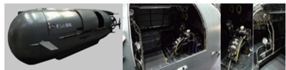
图 6 SUB Seal 湿式蛙人输送艇外形及内舱电子部件布置 Fig. 6 External and internal cabin electronic components of wet diver delivery vehicle SUB Seal
