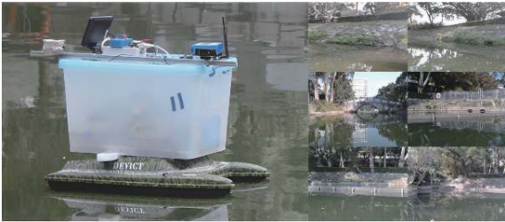
图 5 基于单目视觉的无人艇轨迹跟踪任务 [68] Fig. 5 The USV trajectory tracking task based on monocular visual servo [68]
