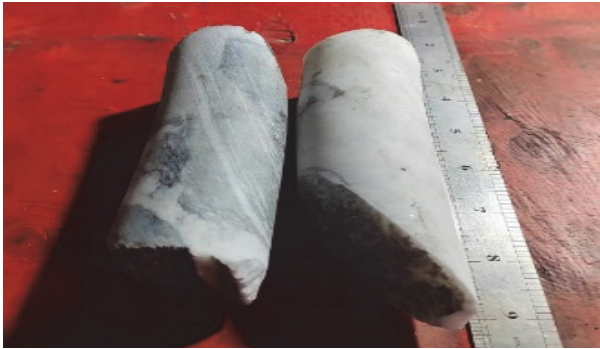
图 4 超深大角度曲线定向钻孔曲线段岩心 Fig.4 Ultra deep curve directional drilling curve section core
