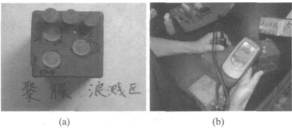
图 8 聚脲粘结力及厚度测试 Fig. 8 Test of adhesive strength and thickness of polyurea elastomer
