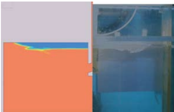
Fig. 10 - The case with a 2 cm silicon oil layer. The simulation displays the same characteristics as the experiment, including the formation of folds and the uncovering of the narrow end of the water.
