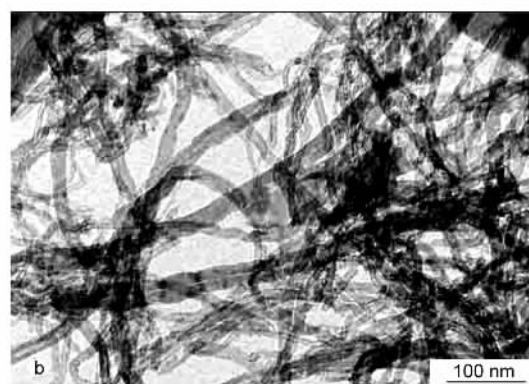
图6 乙醇燃烧产物的 TEM 形貌(a)低碳钢(Bar = 1 μm),(b)含镍合金钢(Bra = 100 nm)
