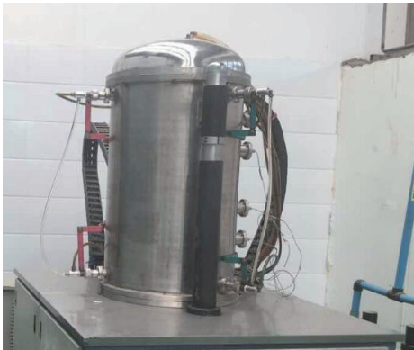
图1 自主研发的ZnS沉积设备 Fig.1 Self developed ZnS deposition equipment
