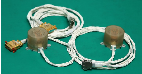
图9 (网络版彩图)磁场探测仪传感器探头实物图 Figure 9 (Color online) Mars rover magnetometer probe physical picture.
