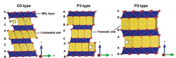
图2 O3、P3、P2型层状K<sub>x</sub>MO<sub>2</sub>晶体结构示意图<sup>[21]</sup> (网络版彩图)Figure 2 Crystal structures of O3, P3, and P2-type layered K<sub>x</sub>MO<sub>2</sub><sup>[21]</sup> (color online)
