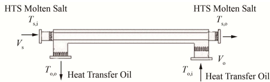
图 2 实验段示意图 Fig.2 Schematic diagram for heat transfer region of test section.
