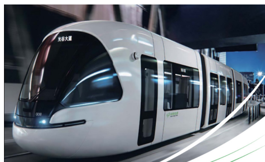
Fig. 11. All-electric tram with ECs of Shanghai Aowei Technology Development Co., Ltd. The energy storage unit can provide 300 A continuous charge/discharge current and 510 A maximum charge/discharge current [63].
