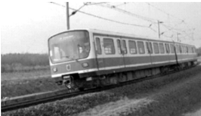
图6 装载直接传动转向架的试验列车 Fig.6 Vehicle with direct drive bogie
