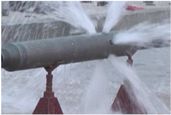
图 15 无限级滑套地面实验开启瞬间 Fig. 15 Opening moment of non-limited sliding sleeve ground test
