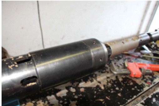
图 14 模拟含砂工况下的滑套开关实验 Fig. 14 Test of sliding sleeve switch simulating under working condition with sand
