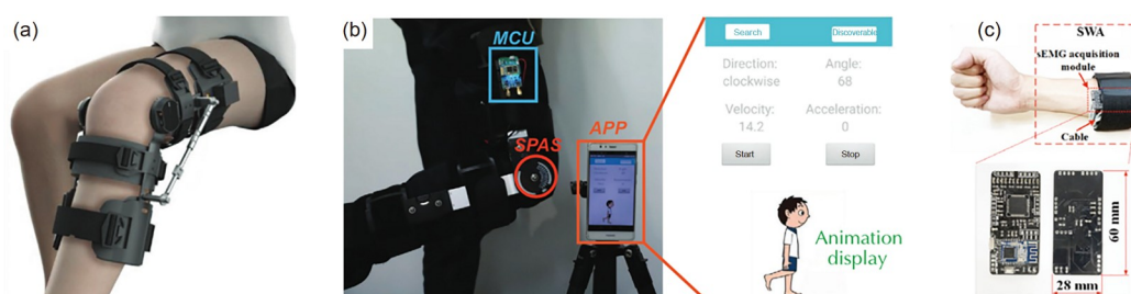
图6 (网络版彩色)运动康复监测与诊断。(a) 可穿戴康复支具系统 [51] 。(b) 角度传感器记录关节屈曲/伸展角度 [52] 。(c) 智能可穿戴臂章 [53] Figure 6 (Color online) Exercise rehabilitation monitoring and diagnosis. (a) Schematic diagram of a rehabilitation brace system [51] . (b) Angle sensor records joint flexion/extension angle [52] . (c) Smart wearable armband [53]
