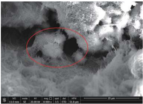
图 6 MPC泡沫混凝土水化产物微观形貌 Fig. 6 Microstructure of MPC foam concrete hydration products
