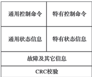
图 6 通用无线通信协议构架 Fig. 6 General wireless communication protocol architecture
